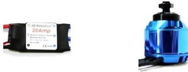
Figure 3.7: 20 Amp ESC (left) and brushless motor (right)
